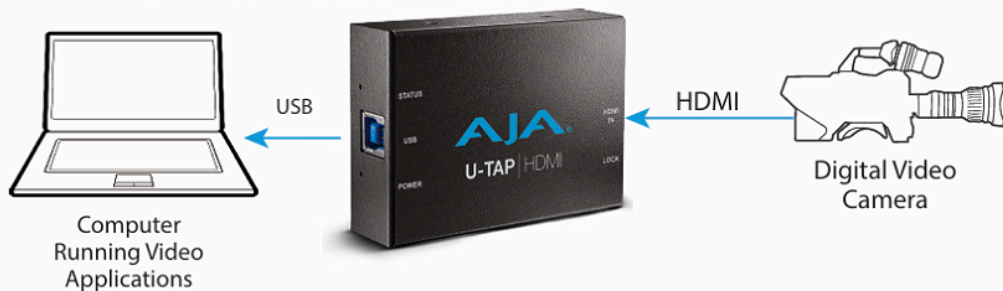
Figure 6. Typical U-TAP SDI Laptop System Connections
